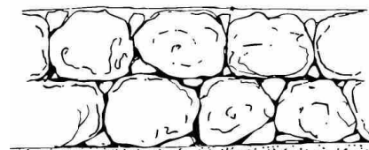
Figure 5: Breaking the joints
